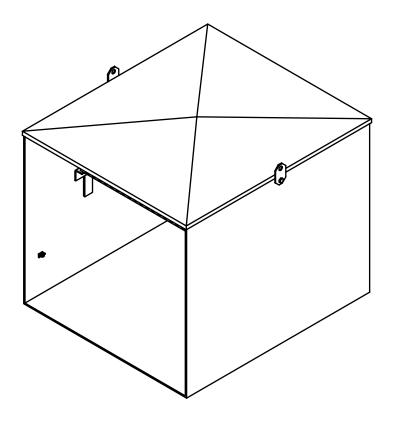
MATERIAL ENCLOSURE: ALUMINUM CONNECTORS: ALUMINUM
